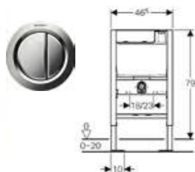
Geberit Duofix frame for wall-hung toilet, 79cm, with low-height furniture cistern
